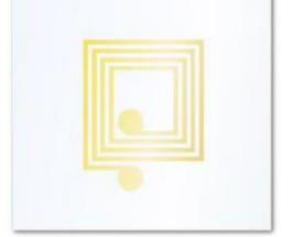
Wei Bo Associates WQL-300 series of spiral inductors feature proprietary photolithographic process and plating techniques on a rugged quartz substrate. This results in a highly repeatable unit to unit inductance value and eliminates hand forming of wire wound inductors and epoxy staking of coils in a hybrid assembly.
